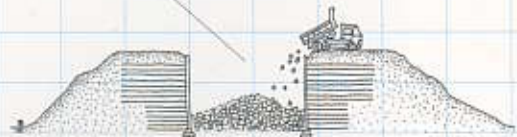
貯蔵堰・防爆壁・堤防
